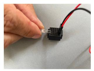
Bend the LED light 90 degrees. Test if the light turns on.
