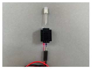
Insert the plug into the bottom of the breadboard. The red cable goes in the row where 1 is marked, and the black cable in the row where 2 is marked.
