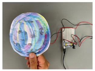
Test if the planet works by inserting it into the larger breadboard. The red cable must align with the red stripe.
