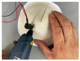
Attach the breadboard with a drop of hot glue. Help the students when working with the glue gun.
