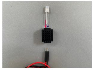
Insert the longest pin of the LED light into the top of the row where 1 is marked. The shorter pin goes to the right in the row where 2 is marked.
